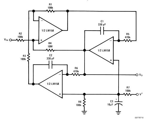
$f_0 = 1 \text{ kHz}$  Q = 50  $A_V = 100 (40 \text{ dB})$
