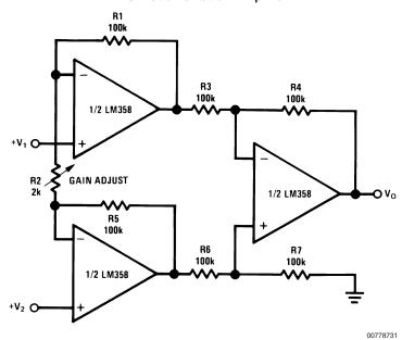
If R1 = R5 & R3 = R4 = R6 = R7 (CMRR depends on match)  $V_O=1+\frac{2R1}{R2}\;(V_2-V_1)$  As shown  $V_O=$  101 ( $V_2-V_1$ )
