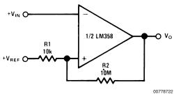
$I_O = 1$  amp/volt  $V_{IN}$  (Increase  $R_E$  for  $I_O$  small)
